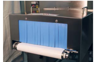
Hygienic design through chamfered surfaces
